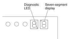
Figure 72. Numeric display LEDs
